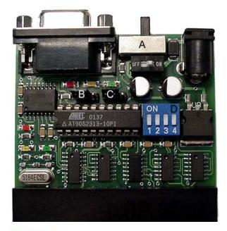
With the host computer system and the USCT turned OFF, locate a free 9-pin serial port on the rear of the host computer system. Connect the FEMALE end of the DB9 cable to the host computer system and the MALE end of the DB9 able to the USCT. Now, connect the power adapter to the USCT and turn the host computer system ON.
